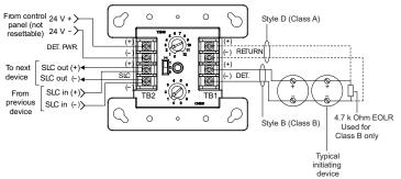
The E-2WIRE can be set for Class B or Class A operation using the slide switch located on the front of the module.
