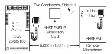
Remote Microphone Panel Dimensions: 8" H x 10" W x 3" D (203 mm x 254 mm x 76 mm)
