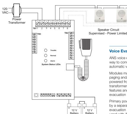
Class B circuit shown. Return wires to evacuation panel for Class A operation.
